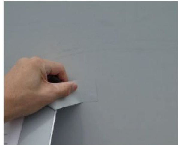
Tedlar® Colored Film vs. Installed Tedlar® after 34 years
